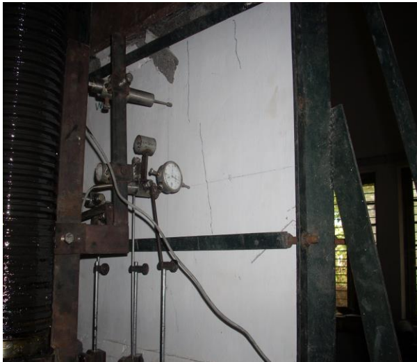
Fig. 4(b). Crack pattern for the specimen WP45
