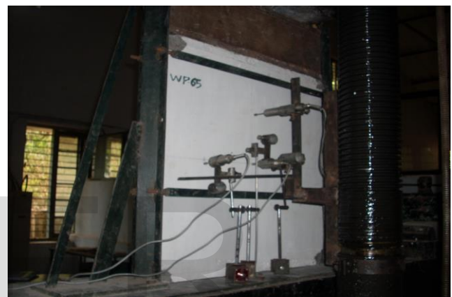
Fig. 1(a). Set-up for lateral deformation
