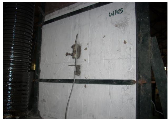
Fig. 1(b). Set-up for vertical strain
