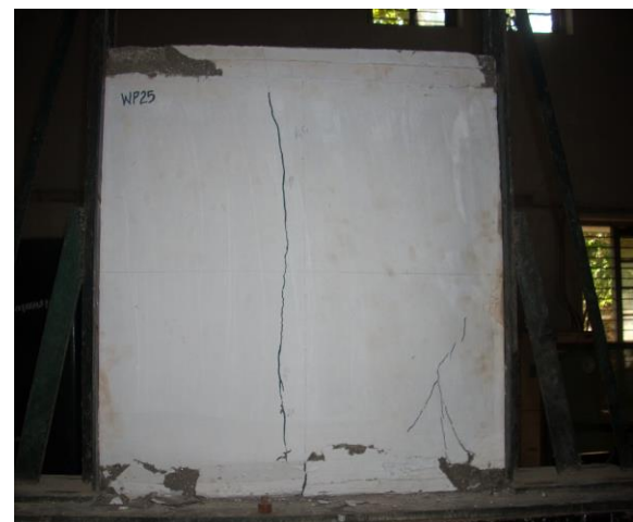
4(a). Crack pattern for the specimen WP25
